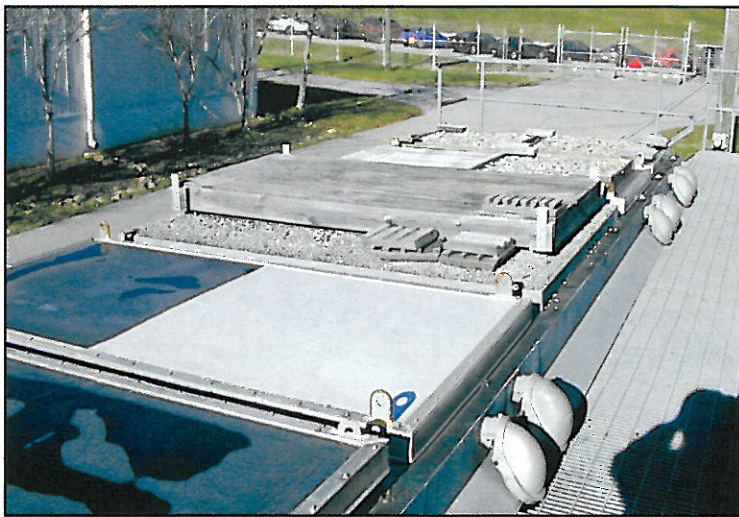
The Roof Thermal Research Apparatus at ORNL configured for ballasted-system analysis.
